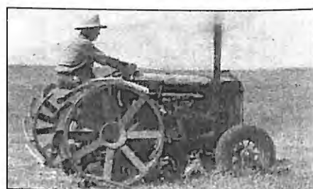
An Australian-made McDonald tractor cutting pasture in the 1950s. Although rubber tyres were released in Australia in 1934 steel wheels were still sold on new tractors well into the 1950s.
