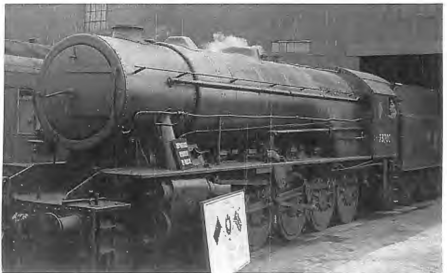
A WD 2-10-0 Class 9F number 73700 at the Mechelen Railway Workshops in Belgium. The small sign resting on the steam pipe states "100th WD loco repaired by "155 RWC RE". The larger sign resting against the piston valve gear states "155 RWC RE". Followed by their motto "EX Nihil Venit Omnia" (From nothing came everything), and underneath the Railway Workshop Company's emblem appears a list of the places where the men of 155 Company were associated. (Teheran, Baghdad, Ahwaz, Swindon, Wolverhampton, Mechelen, Eastleigh, Ashford, Derby, Crewe, Bow, Doncaster, Darlington, Stratford, Rennes and Dieppe).
