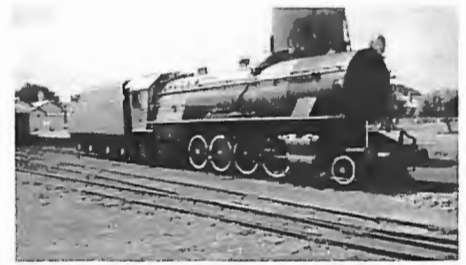
Class V 2-8-2 number 1209 built in 1955 by Robert Stephenson & Hawthorns Company under licence from Beyer, Peacock & Company for export to Australia, and now operating on the Bellarine Peninsula Railway in Victoria
