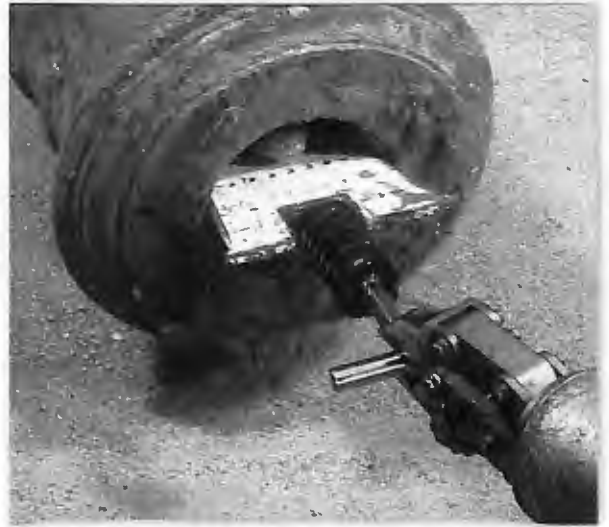
Scientific: A robot arms measures the bore hole of a bronze cannon.
