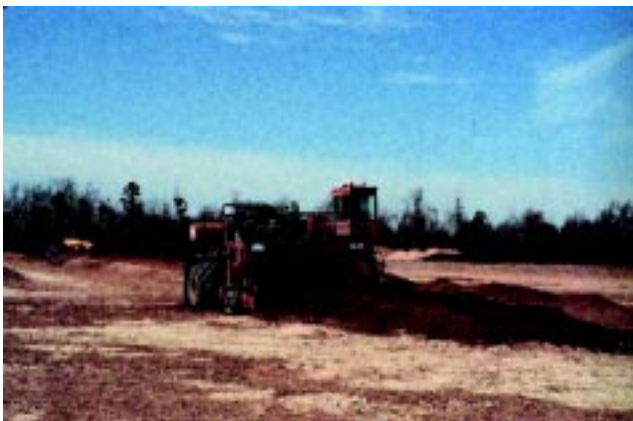
Figure 6c. Turning poultry litter using a self-propelled windrow turner
