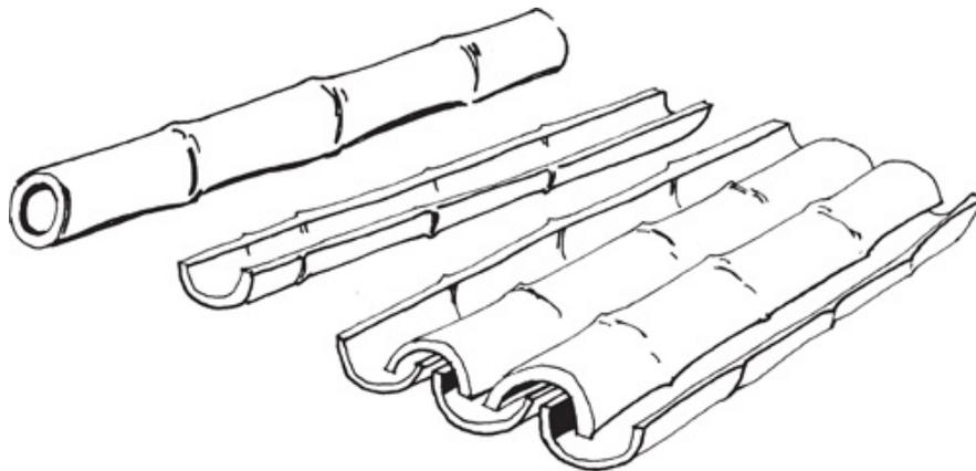
*Split bamboo vertically to make roofing and guttering to collect rainwater. The split stems, laid alternately to interlock with one another, form efficient and waterproof pantiles.*
