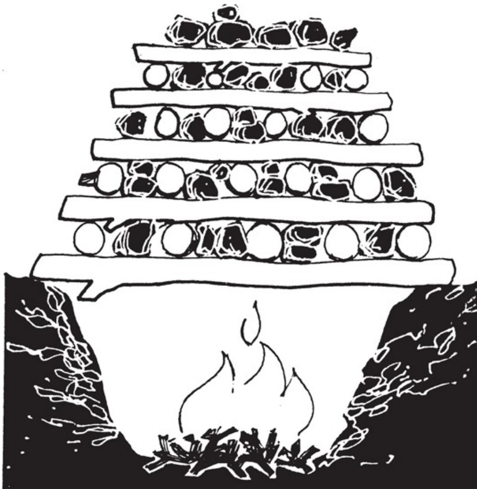
*Dig an oval-shaped hole with rounded sides 45–60cm deep (18–24in) and place kindling at the bottom. Lay logs across the hole, place another layer of logs at right angles to them, interspersing them with stones. Make another layer of logs and build up five or six more alternating layers, topping them off with stones.*
