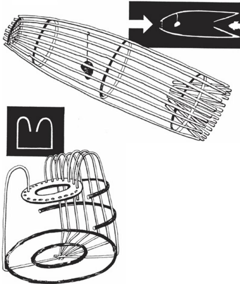
*The torpedo shape is made from wicker woven and tied in position. Place the opening downstream, against the current. The entrance starts quite wide, making it easier to enter, but inside the angle of the struts makes escape difficult.*
