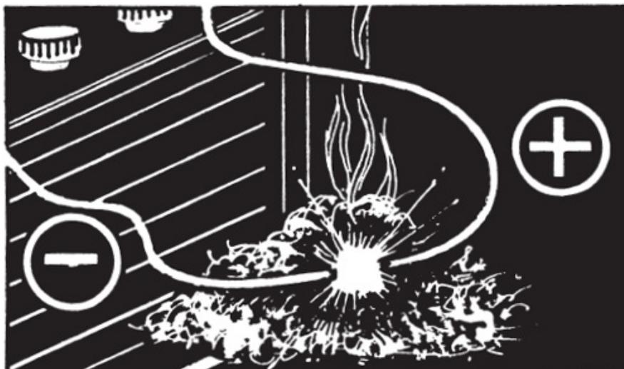
*Slowly bring the bare ends of the two pieces of wire together. Just before they touch, a spark will jump across. You must catch it on your tinder. A small piece of cloth with a little petrol on it makes the best tinder, the petrol vapour igniting from the spark.*
