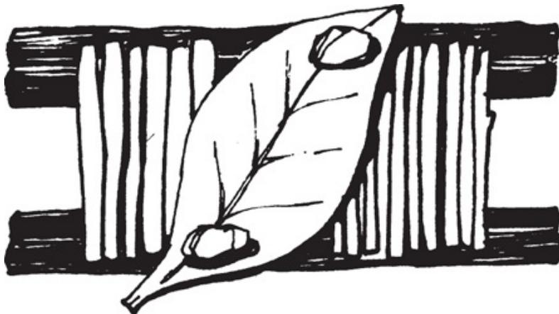
*Make a lid of smaller wood to cover the opening or use a large flat rock or a large leaf weighted down with stones. Always remember to replace it.*
