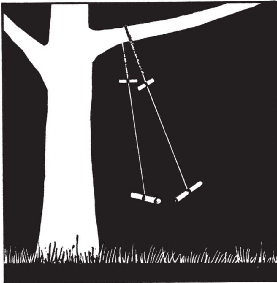
*Very high branches can be removed by attaching strings to the saw toggles to give extra reach. This is dangerous. Keep your eye on the branch and be prepared to jump out of the way.*
