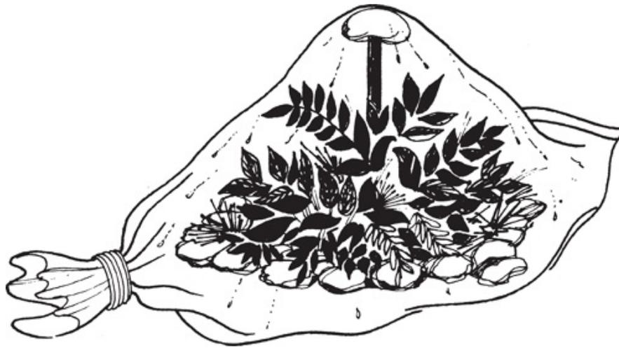
*Even cut vegetation will produce some condensation as it warms up when placed in a large plastic bag. Keep the foliage off the bottom with stones so that water collects below it, and keep the foliage from touching the plastic. Use stones to keep the bag taut. Support the top on a padded stick. Arrange the bag on a slight slope to encourage condensation to run down to the collecting point. When no longer productive carefully replace with fresh foliage.*
