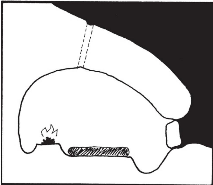
*Smooth the inside surfaces to discourage melt drips and make a channel around the internal perimeter to keep them away from you and your equipment.*
