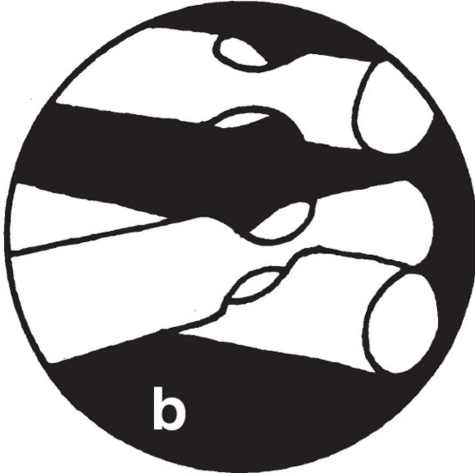
Lay down your first layer of logs in the shape of your hut (a). Joint the corners to fit on top of each other (b) and cut other logs to fit neatly on top.
