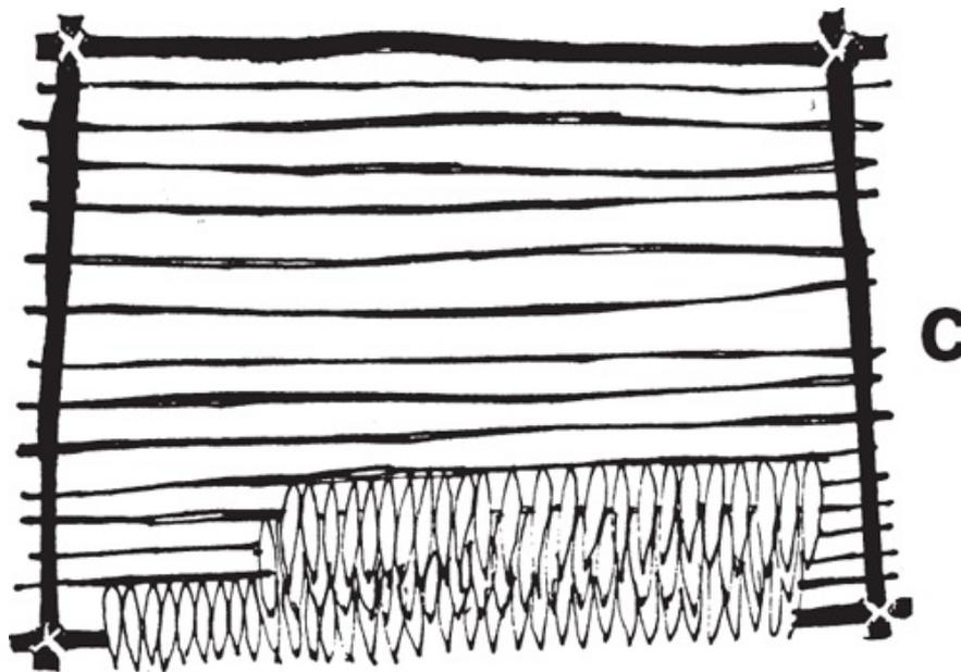
*Closely layer halves of atap on your roof frame (c). You can let it be a little less dense on walls. Woven atap can be particularly effective for the sides of a shelter.*
