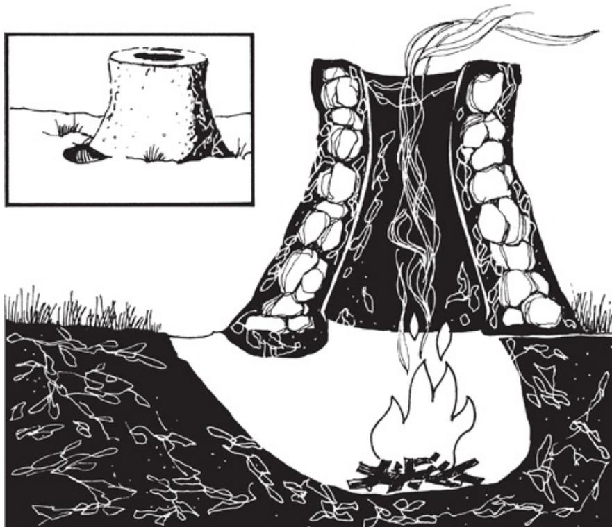
Dig a hole circular in shape and about 24cm (9in) deep with a channel on one side leading down to it. Set rocks up all round the outer edge of the main hole and build up a funnel, bridging over the channel and gradually sloping inwards. Let the upper courses begin to open out again. Seal all the spaces between the rocks with earth. The fire is shielded, the chimney creating a good draught.
