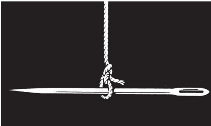
*Suspend the needle in a loop of thread, so that it does not affect the balance. Any kinks in or twisting of the thread must be avoided.*
