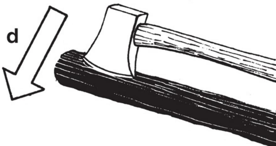
Alternatively, hold smaller log against cutting edge of axe and bring both down together (d) on to a larger log. (Not to be tried holding too short a log for safety.)
