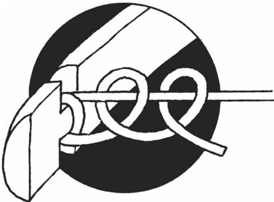
*Secure the string to the bow with a round turn and two half hitches at each end. If the wood is unseasoned release one end of the string whenever the bow is not in use to relax the tension or you may find the stave sets in shape.*
