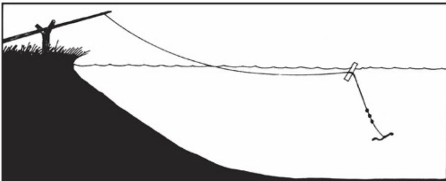
A deeper hook position can be ensured by extending the line to a weight below the hook.
