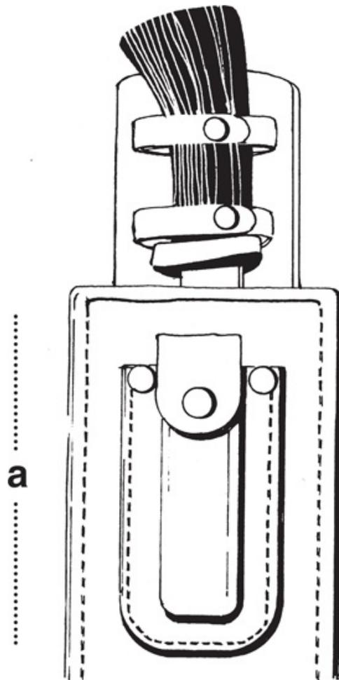
The sheath must have positive fastenings to keep the parang secure, and a loop for fixing to a belt. Some sheaths have a pocket on the front for a sharpening stone.
