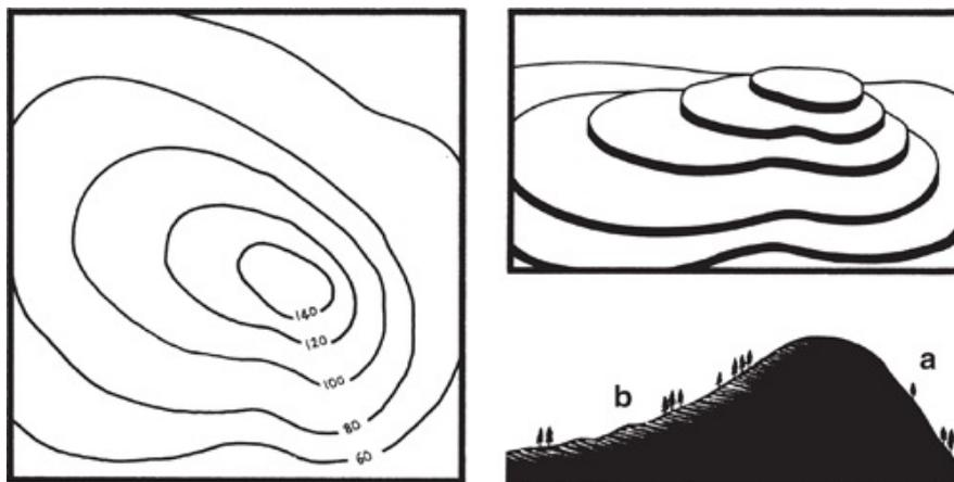
*The contour lines on the map represent a series of points at the same distance above sea level and do not record what happens in between. When the contours are closely grouped the change in height is more rapid (a). Conversely, greater spaces between the contour lines indicate gentler slopes (b).*
