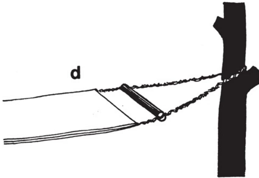
*Insert spacer bars, notched at each end (d) to take the lines and tie your hammock to two convenient trees or stout posts.*
