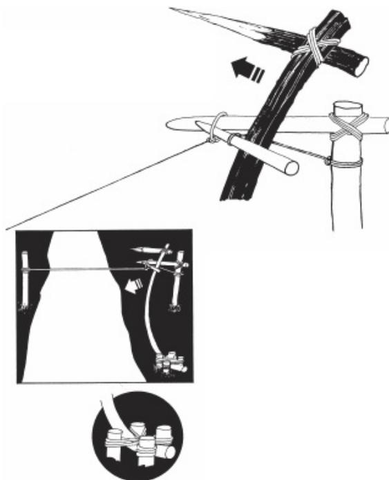
(a) Notch arrow for bowstring and for trigger bar. Angle trigger bar tip to fit arrow notch, cut side to fit cross-bar. Sit toggle between bottom of trigger bar and a fixed post.
