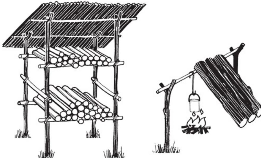
*Rest logs against a pot rail to dry. Build a wood shed — essential in wet weather. Set it close to the fire so that the fire's warmth will help dry the wood, but not so close that a spark could ignite it. Build two bays and use wood from one while the other batch dries.*
