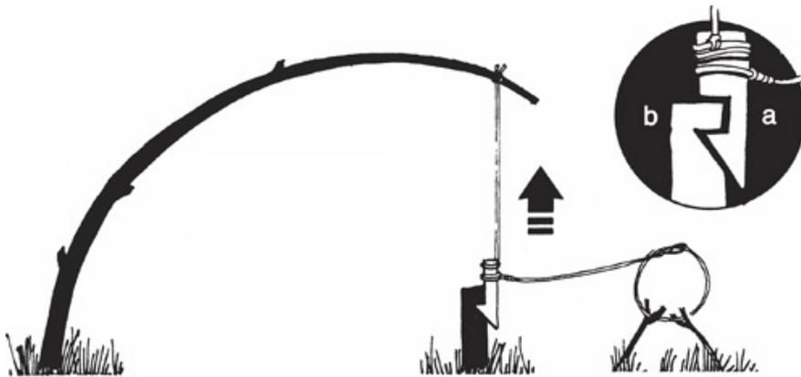
*Cut notch in trigger bar (a) to fit notch in upright (b). Drive upright into ground. Attach snare to trigger bar and use cord to sapling to keep tension.*
