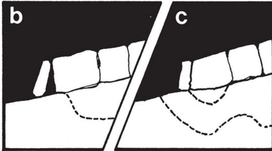
*Block the windward end with another block or piled up snow. At the other end (downwind) have a removable block as a door (b), or dig an entrance (c). Fill any gaps with snow. Most effective built on a slight slope, cold air will collect in the entrance leaving warmer air in the sleeping space.*
