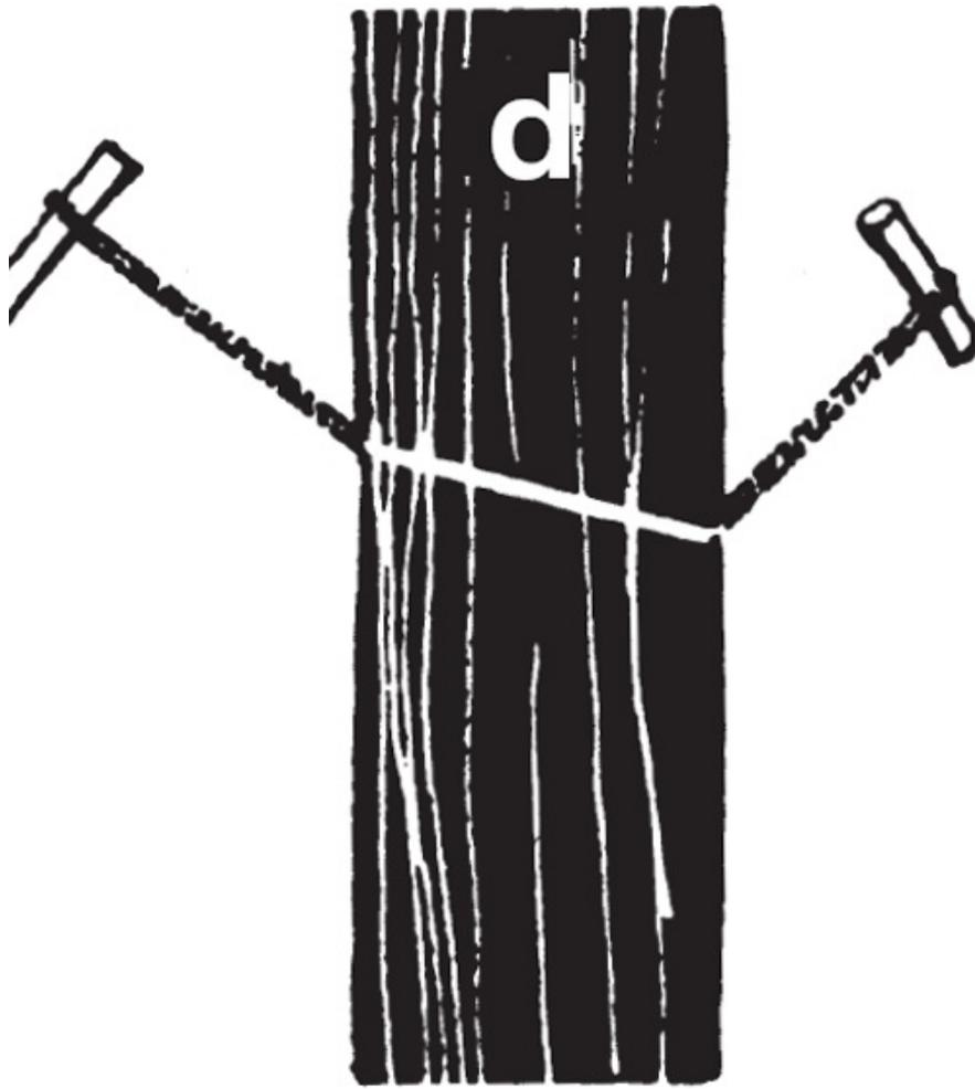
*At all times keep the wire taut (c) pulling in a straight line, never at angles (d).*
