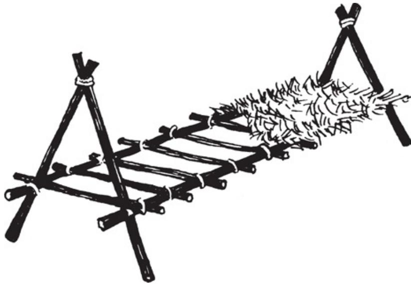
*Lash the end 'rungs' to the A-frames, jutting out either side. Make these of strong timber and lash them securely. Fit the ladder over the frames and lash in place. Lay bedding of bracken, ferns or leaves.*
