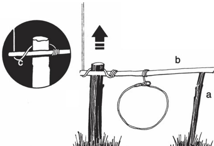
*Note how the switch line secures one end of snare arm (b), while the other rests on the keeper stick (a). Keep the switch line near the end of the snare arm (c).*
