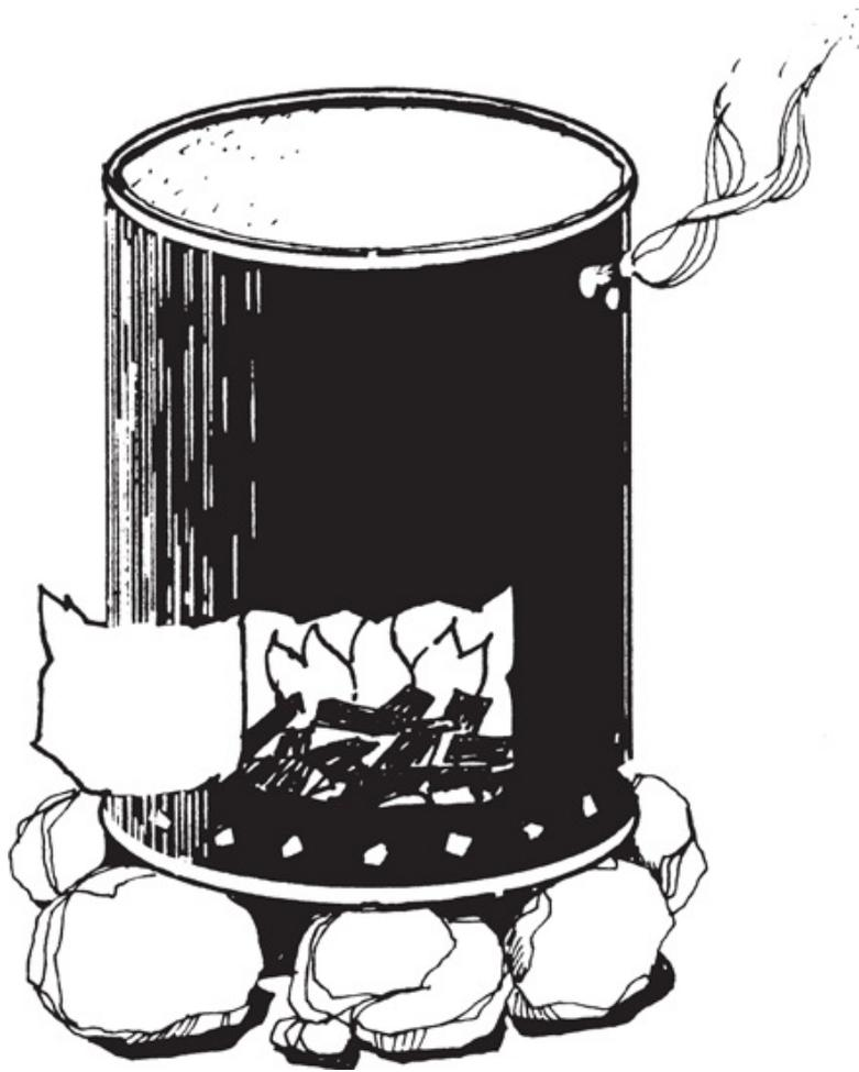
*Punch holes in the bottom and around the bottom of the sides of the drum for draught to enter. Cut out a panel on one side, about 5cm (2in) from the bottom through which to stoke the fire.*
