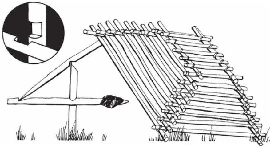
Experiment with different ways of making a cage. You may have a suitable box or large tin which would do just as well. It is also possible to prop the raised edge of the cage on a single stick tied to a long line. Take the other end of the line and hide some distance away. If you hold the string taut, you can snatch the prop away as soon as a bird ventures under the cage. Broadcast bait around and under the cage. This works best in areas where birds seem plentiful.
