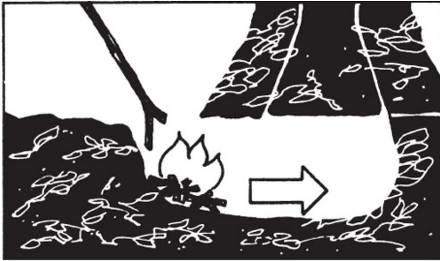
*Light the fire first in the channel. When it gets going push it beneath the chimney. Fuel is then fed in through the top of the chimney and the rate of burning is controlled by opening or closing the top.*
