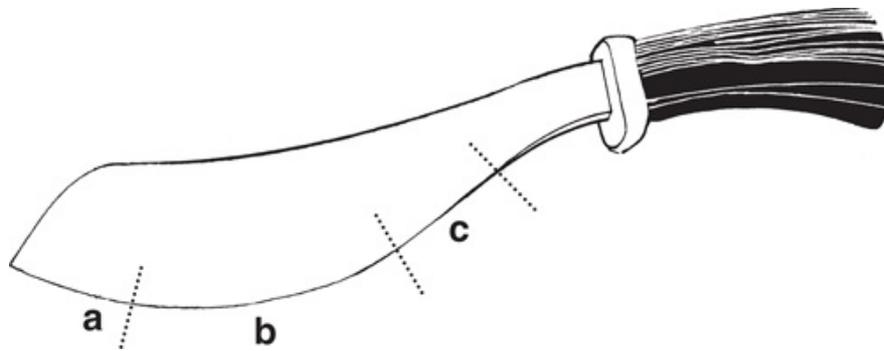
The parang blade has three different edges: **b** does the heavy work of chopping wood and bone, **a** is finer and used for skinning, **c** is finer still for cawing and delicate work. **a** and **c** are easily maintained and **b** is sharp but not so sharp as to chip easily.
