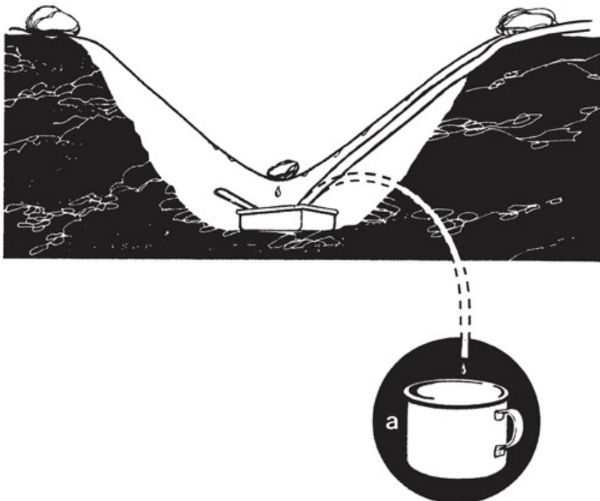
*Roughen underside of sheet with a stone to ensure droplets run down it. Use stones or weights to secure edges and keep cone shape. Fix can so that trapped creatures cannot tip it over.*
