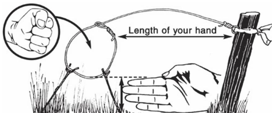
*A wire snare (as big as your fist) can be supported off the ground on twigs, which can also be used to keep a suspended string noose open.*
