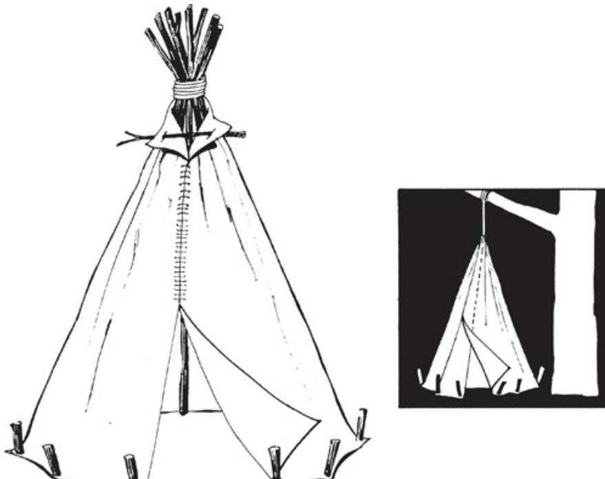
*Parachute material can be used to cover a tepee, but even simpler is to suspend one from a tree. Give the sides a steep angle and, even when the fabric is not impervious, water will run off. Fold a segment of the chute double for a door flap, slit along a seam and make a tie fastening to close it.*
