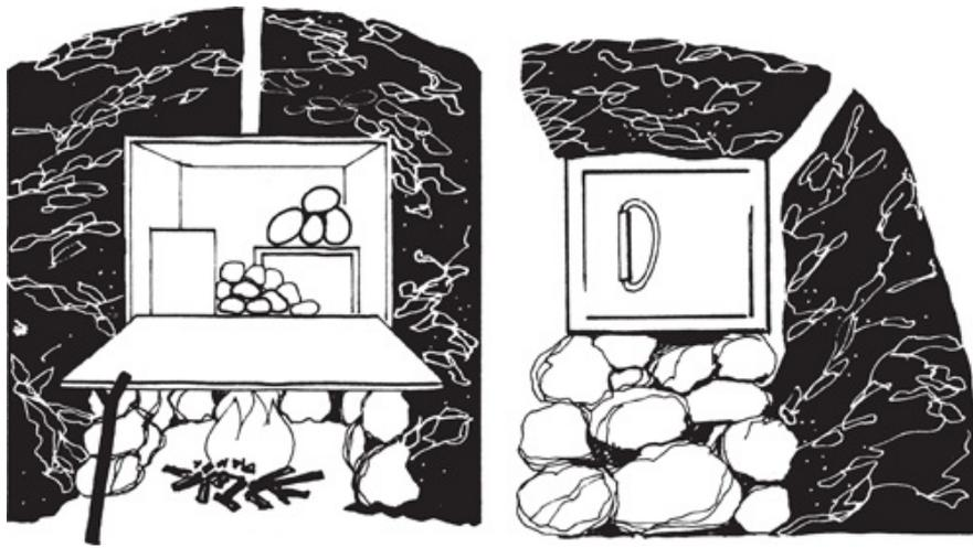
*Stand the tin on some rocks so that a fire can be lit beneath it. Build up rocks and earth — or, better, clay — around back and sides and over it, but leaving a space behind for heat and smoke to move around the back. Use a stick to make a chimney hole from above to the space at the back.*
