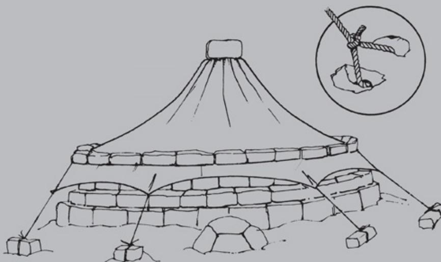
*Anchor parachute cords with further blocks of ice or snow or cut a hole in the ice and pass the rope through it to make a firm anchorage.*
