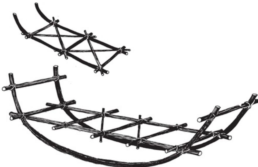
*Choose two forked branches and remove one side of each fork. Make smooth for the runners and lash on cross members. Alternatively, choose two longer supple runners. Bend and brace as shown. This arrangement keeps the lashings off the ground and may be more comfortable for an injured person. Whichever method you use, add at least one diagonal for strength.*
