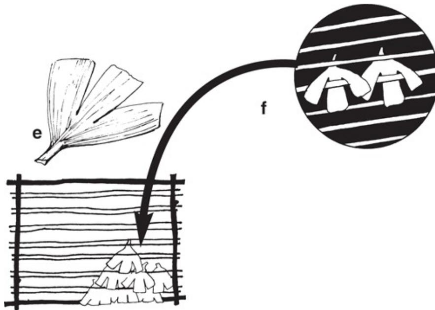
Three-lobed leaves or leaves cut in this fashion (e) can be locked over a thatching frame without any other fixing being necessary to hold them in place (f).
