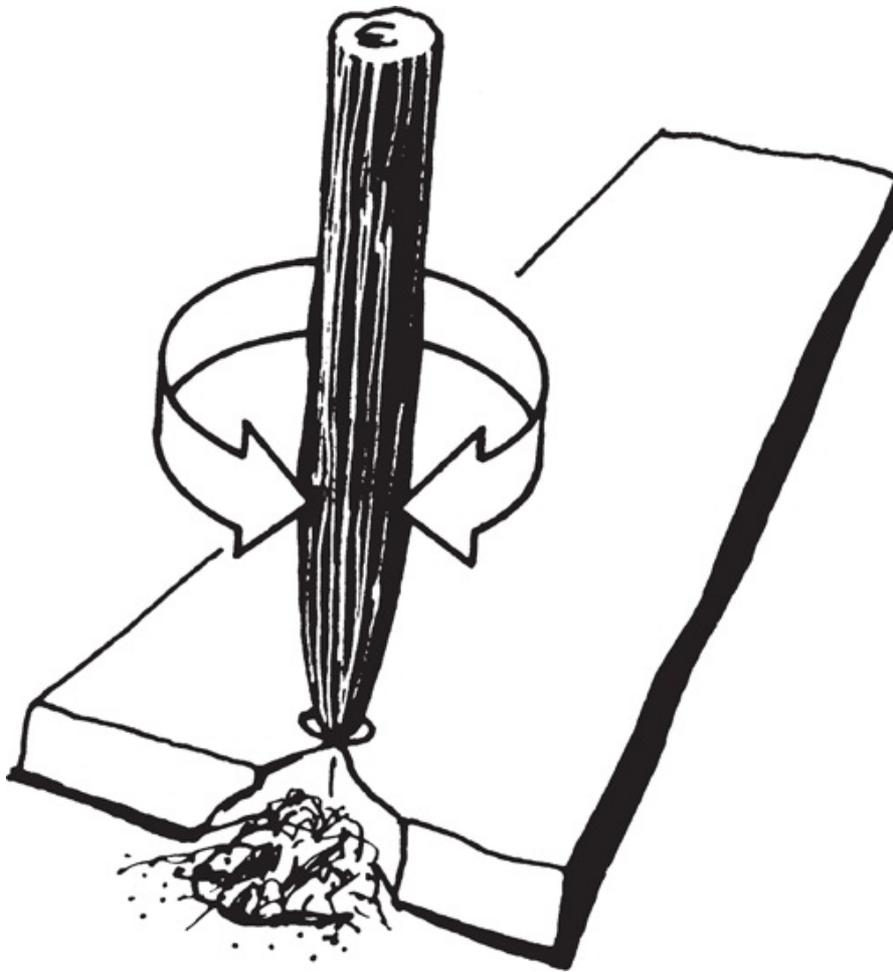
*In a baseboard of hardwood cut a V-shaped collecting notch which will hold tinder, but still allow air to reach it. Make a small depression near it. For a spindle use a stem of hollow softer wood with a soft pith core.*
