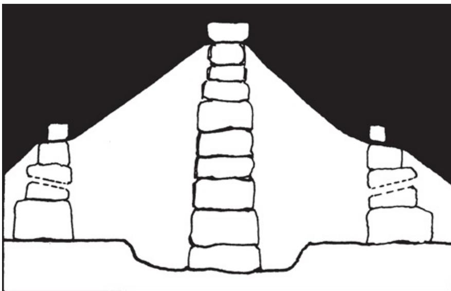
*Raise a central column of blocks in the centre about 1–1.5m (3–5ft) higher than the wall. Drape the parachute over this and the wall, securing it with a further row of blocks on top of the wall.*
