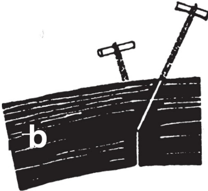
**USING A FLEXIBLE SAW** Always use a flexible saw so that the cut opens up (a) rather than closes tight (b) on the saw, causing it to jam. Do not pull too hard or the saw may break.
