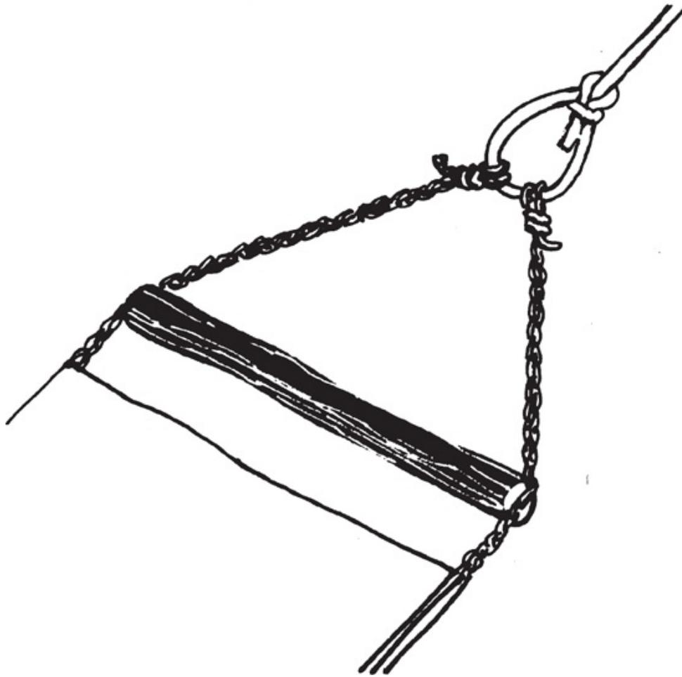
*If you have another piece of rope, or plait some from unused rigging lines, you could tie both the hammock strings to a fixed loop, such as a bowline (see Knots). Experiment with different ways of suspending your hammock, until you find the most stable and comfortable.*
