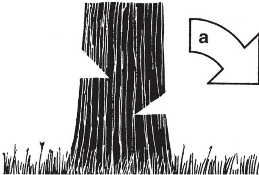
*Cut from both sides of the tree, first chopping out a notch at an angle of about 45 degrees and another on the opposite side at a lower level, ON THE SIDE TO WHICH YOU WANT THE TREE TO FALL (a). Do not cut through more than half the tree before starting the other notch.*
