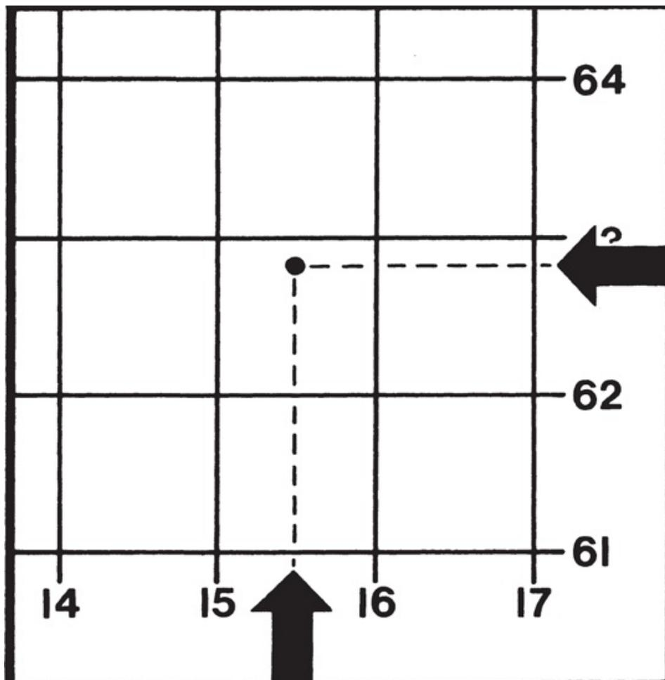
*The point marked with a dot can be described as 15.5 x 62.8 using the coordinates from the sides of this grid. This system requires that squares are mentally divided into tenths in each direction. The 'map reference' is normally expressed as six digits: 155628. Any letter area codes on the map should be included.*
