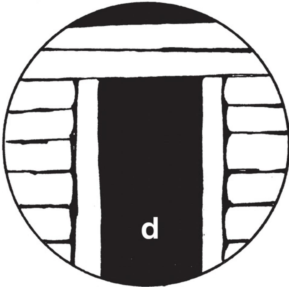
*Once the ground frame is established leave space for a doorway on the side away from the prevailing wind — you may be able to use off-cuts from logs for these sections on either side of the door. Square off the edges and wedge a door frame in place (d). Do not bother with windows, the door will give sufficient ventilation.*
