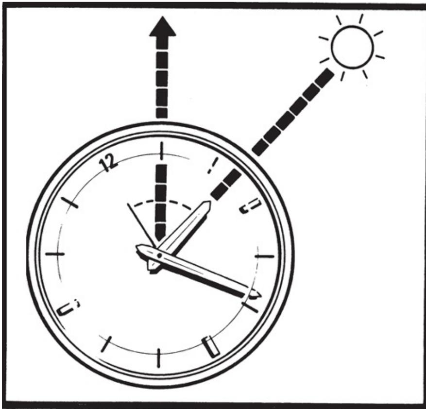
**Northern Hemisphere** Hold the watch horizontal. Point the hour hand at the sun. Bisect the angle between the hour hand and the 12 mark to give a north-south line.
