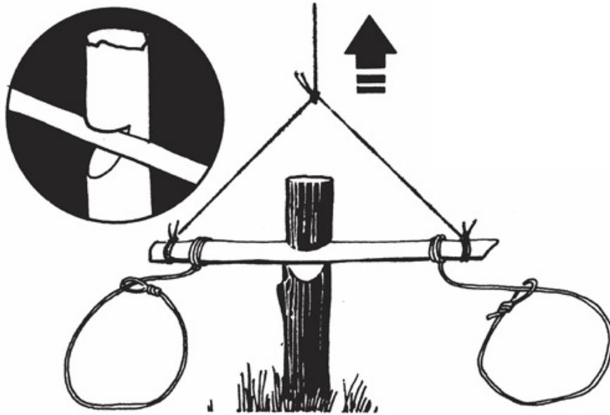
*Once ensnared, the animal's struggles will disengage the snare arm regardless of the direction from which it originally approached.*
