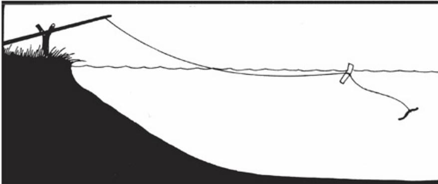
Small weights between the float and the hook will stop the line from trailing along the water or at too near the surface in a current, still leaving the hook itself in movement. You have small split lead shot in your survival kit. Slip the groove along the line and squeeze in to fit closely.
