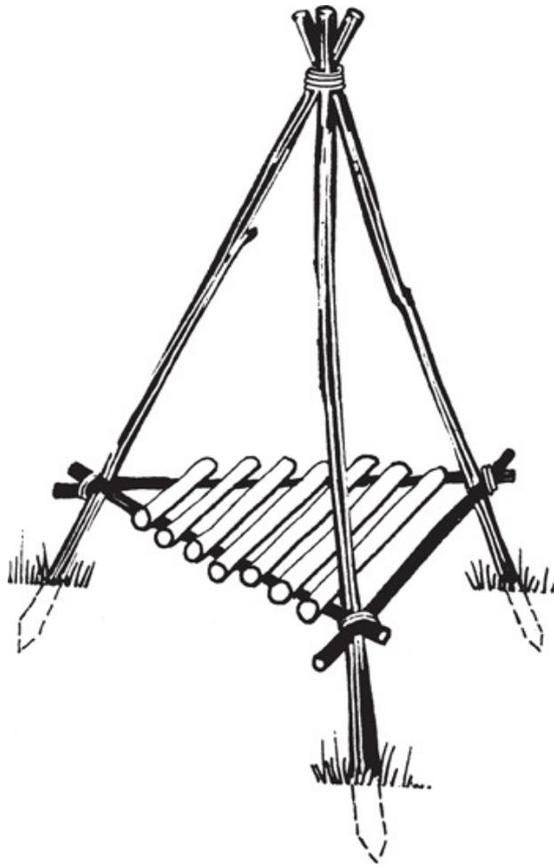
*Keep these tripods well maintained, ensuring that wood is dry enough to light at a moment's notice and that the supply is not poached for other uses. Drive the pole ends into the ground to prevent tipping over in strong winds.*
