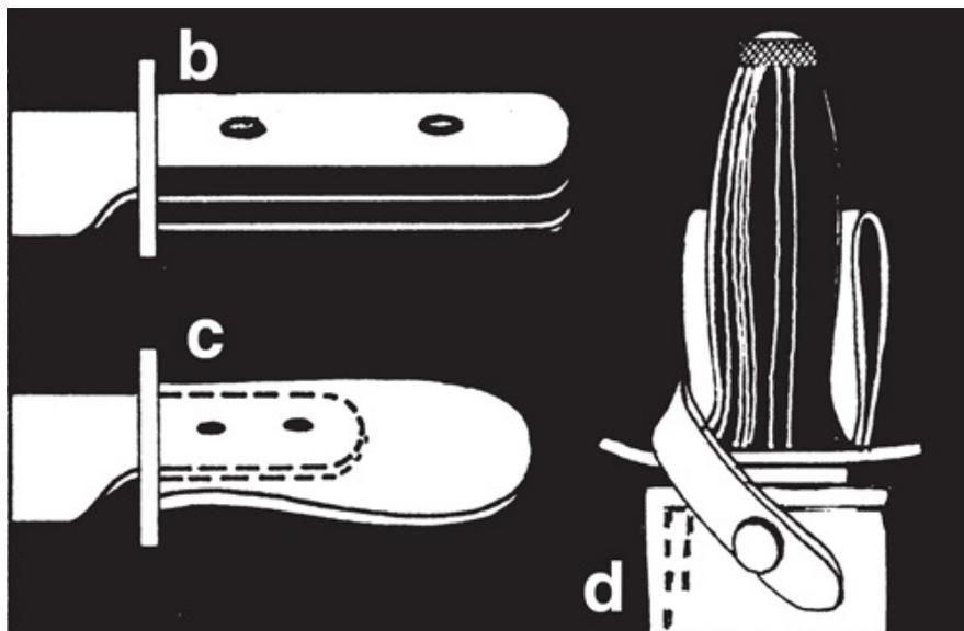
*Handle (a) is ideal: a single rounded piece of wood, the knife tang passing through it and fastened at the end. If the handle breaks the tang can be wrapped with cloth or twine. Handle (b) is only riveted to the tang and would cause blisters. Handle (c) could break at the rivets if subjected to heavy work and the short tang would make it difficult to improvise a handle. The sheath (d) should have a positive fastening and a tunnel belt loop.*
