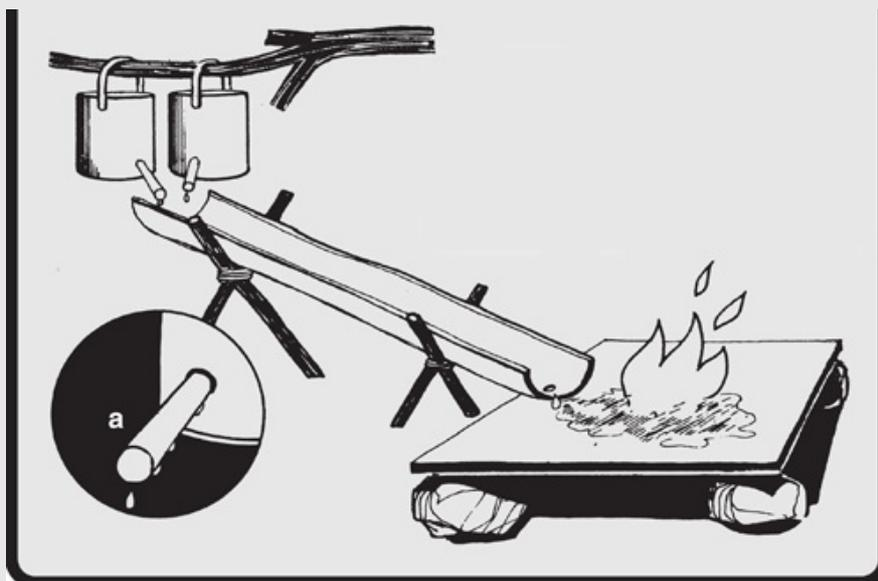
*First light a small fire under the plate to get it hot. The mixture becomes highly volatile when heated. Light it above the plate. This fire will burn almost anything.*
