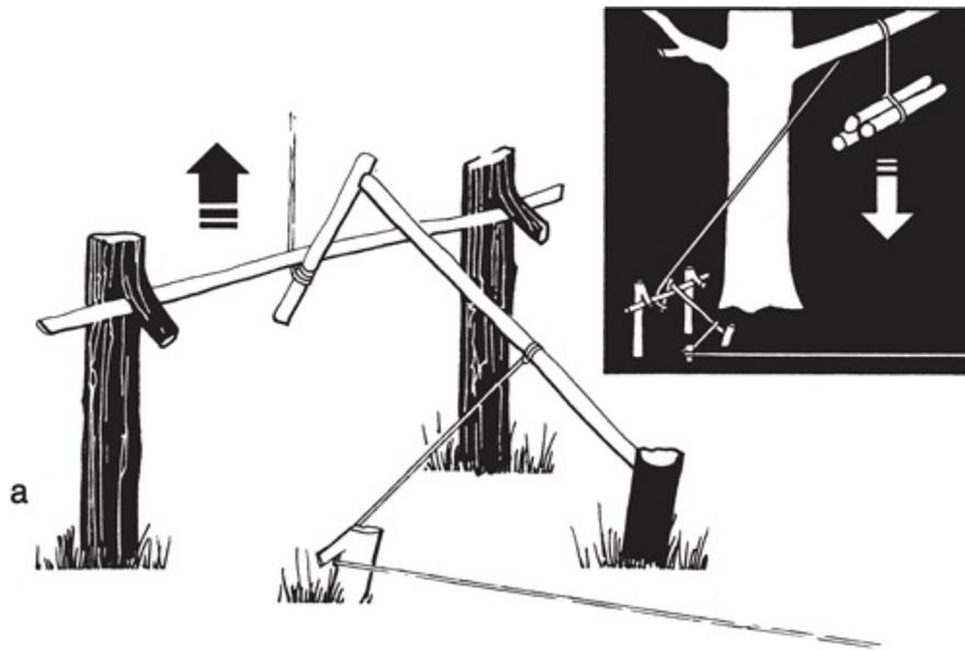
*Run the trip line under a forked stick (a) so that it will pull the trigger bar sideways when operated.*
