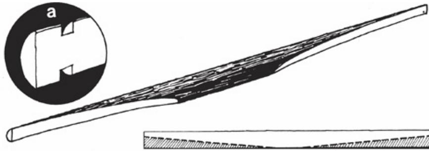
*Fashion the stave so that it is 5cm (2in) wide at the centre, tapering to 1.5cm (5/8in) at the ends. Notch the ends (a) to take the bowstring about 1.25cm (1/2in) from the ends. Remove the bark if you choose. When the bow has been whittled into shape rub it all over with oil or animal fat.*
