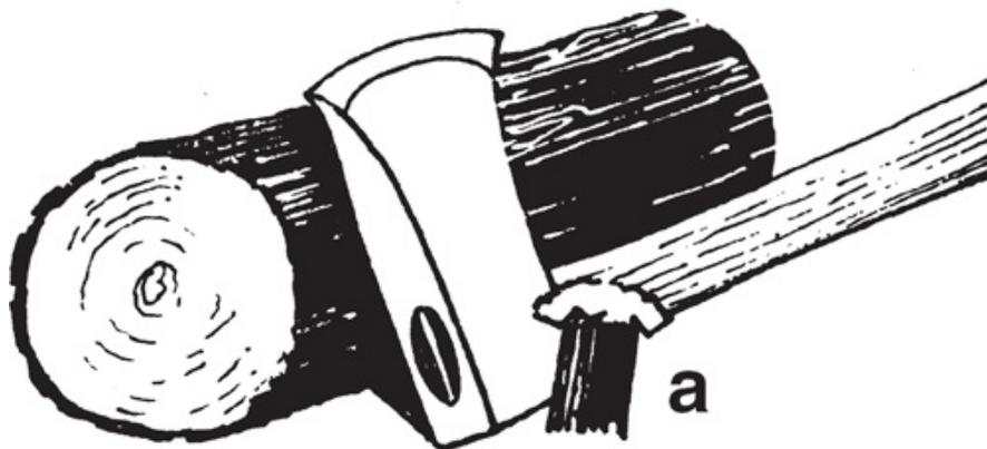
*Prop axehead between a log and a peg (a). Always try to sharpen INWARDS from cutting edge to avoid producing burrs.*
