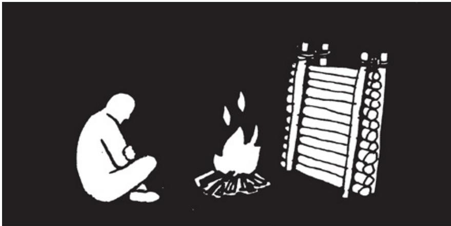
*A good reflector, close to the fire, not only reflects heat back to you but also helps to make the smoke go upwards, drawn by hot currents of air, instead of getting in your eyes. Use a reflector to direct heat into a sleeping shelter.*
