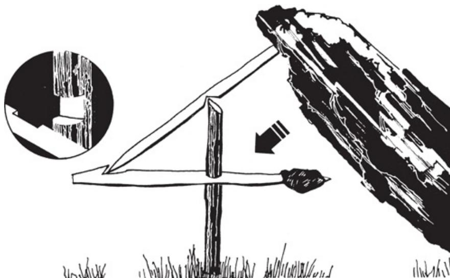
*Bait bar notched on top to engage locking arm, square cut on side to fit upright. Locking arm sharpened at lower end to release quickly, notched at centre to pivot on upright.*
