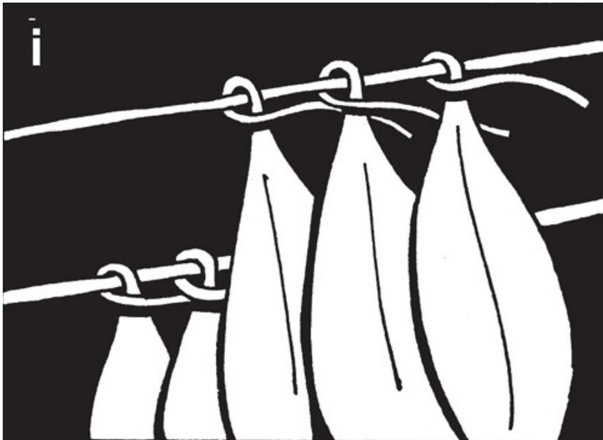
*Palm and other long-stemmed leaves can be secured by carrying the stem around the batten and over the front of the leaf, where it is held in place by the next leaf (i).*
