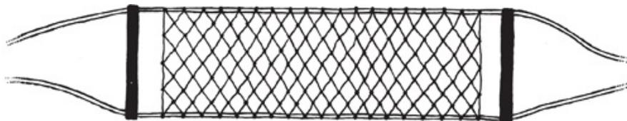
Cut two spacer bars to keep the hammock 'open'. Notch the ends and slip the cords into the notches (a). To simplify hanging the hammock you could tie each pair of end lines to a fixed loop such as a bowline. Then fix one end with a round turn and two half-hitches, the other with a quick-release knot, in case you ever need to leave the hammock in a hurry.
