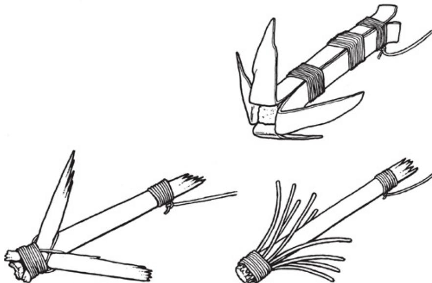
*Make a grapple hook by lashing pieces of wood or metal wreckage together to form a multiple hook. Attach it to a line and trail it behind, or throw it out to rake in weed. You can use it for gathering other drifting wreckage to consolidate a makeshift raft.*
