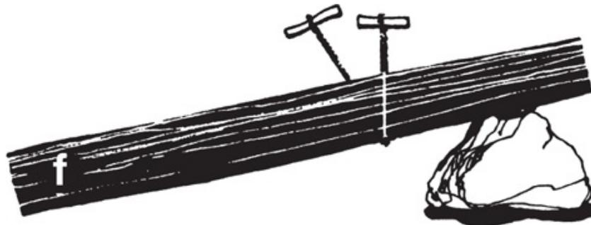
*It is usually easier for a single person to cut a log by pulling upwards (f). Support the log to keep it off the ground and give it an angle to keep the cut open.*
