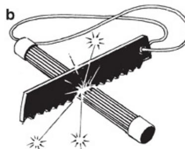
*Strike the blade against the flint (a), or draw the saw across the ridged surface of the flint supplied with it (b), close to tinder so that sparks fall on it.*
