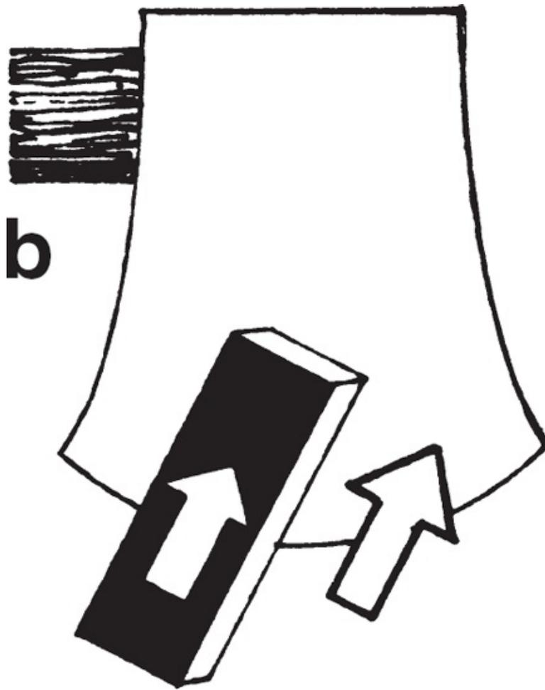
*Use a file or rougher stone first to remove rucks and burrs (b). Then finish with a smoother stone, using a circular motion. Don't drag the stone off the cutting edge. Push ONTO blade. (See [Knives in Essentials](#)).*
