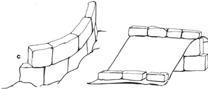
Anchor a ground sheet or poncho along the top with another course of blocks, use others to secure the bottom edge. Use more snow blocks to close the sides.
