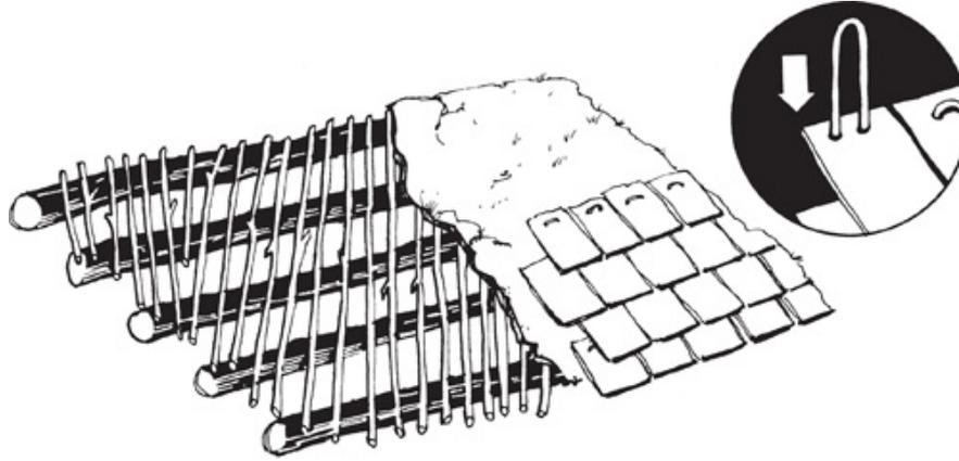
*Instead of a complete roof of whole logs you could use lighter materials and mud on a timber frame. Bark from the logs makes an excellent top covering if laid as tiles. These could be pegged through with small supple twigs while the mud is still soft.*
