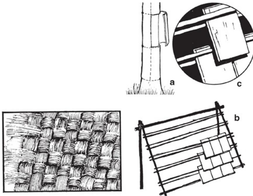
*Long grass can be bunched and woven (overlap the ends irregularly) to make a continuous warp and weft. Or use birch bark to make shingles. Ring a birch tree with even 60cm (2ft) cuts and carefully remove the bark (a). Across a frame fix pairs of canes or creepers in close-spaced pairs (b). Upper ends of shingles are gripped between the canes, the lower ends rest on top of those below (c).*
