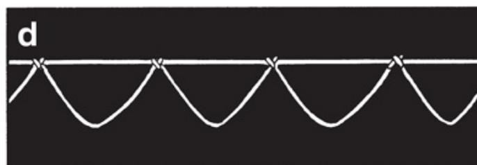
To make the net, tie a top line of required length between uprights. Begin by tying a clove hitch with thinner line (b). Take the needle behind the top line and bring it forward to make another clove
