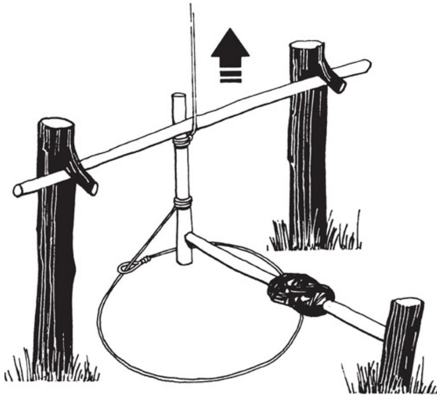
*Taut line from bent sapling to end of toggle pulls against cross-bar. Bait bar keeps toggle in position.*
