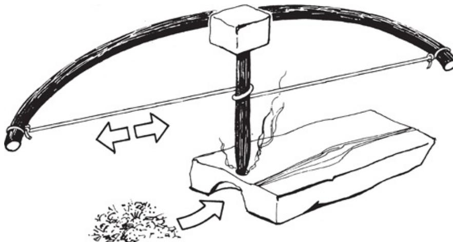
*Keep on bowing until unable to continue. If successful the tip, glowing like a cigarette, will drop onto your tinder, which, if you gently blow on it, will burst into flame. You must keep the spindle upright and steady.*
