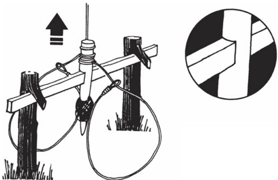
*Retaining bar, or at least a section of it, should be squared off to fit a square-cut notch on the bait stick.*
