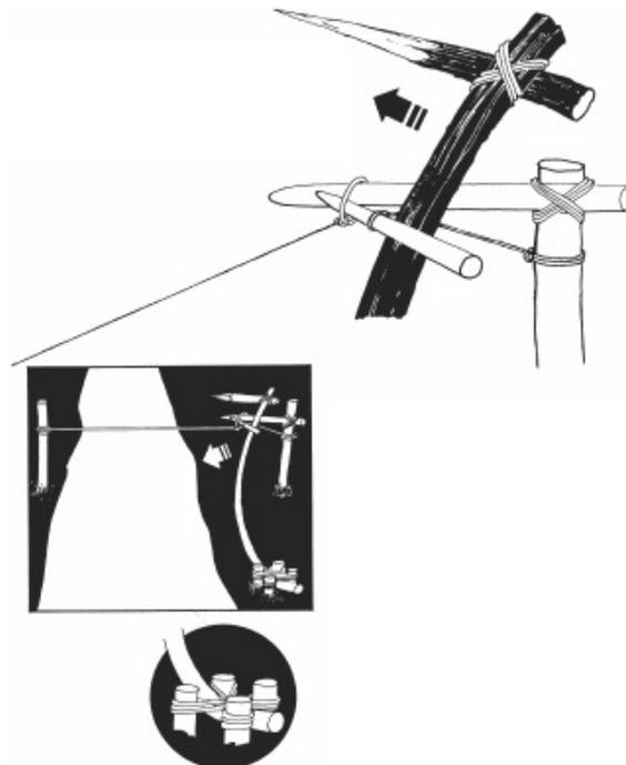
*Make sure that the spear is lashed very firmly to the springy shaft or it may be knocked sideways on impact instead of plunging into the animal's body.*
