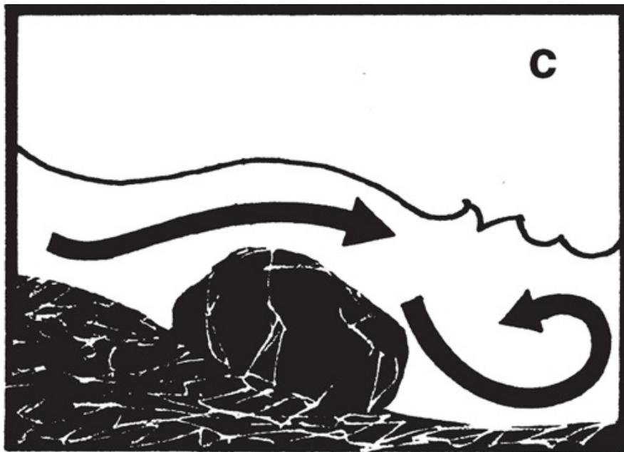
*Closer to the surface an obstruction will create an eddy downstream of it where the surface water appears to run back against the main flow. If a large boulder coincides with a steep drop in the level of the bottom (c) these eddies can produce a powerful backward pull downstream of the obstruction and pull swimmers in — they are VERY dangerous.*
