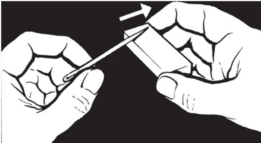
*Stroking with a magnet, should you have one, will be much more efficient than using silk — stroke the metal smoothly from one end to the other **IN ONE DIRECTION ONLY**.*
