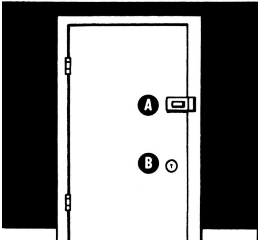
*The rim lock (A) should be positioned one third of the way down from the top of the door. The mortice lock (B) should be positioned one third of the way up from the bottom of the door.*
