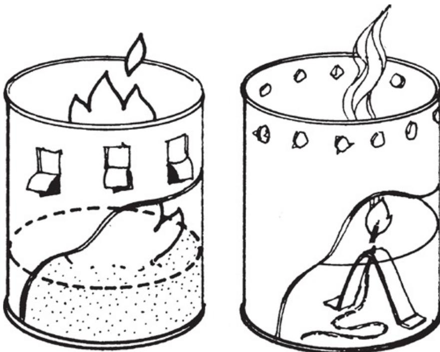
*Mix petrol with sand and burn it in a container as a stove, or dig a hole and make a fire pit.*
