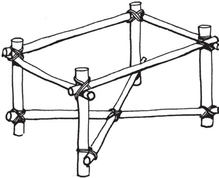
*Make a simple box frame with cross-members linking legs from short lengths of wood. To make a seat: weave vines or twine back and forth or sew on a piece of canvas or plastic with thongs. Failing these, try a flat piece of wood or metal laid across, or thin springy saplings lashed to the frame and interwoven.*
