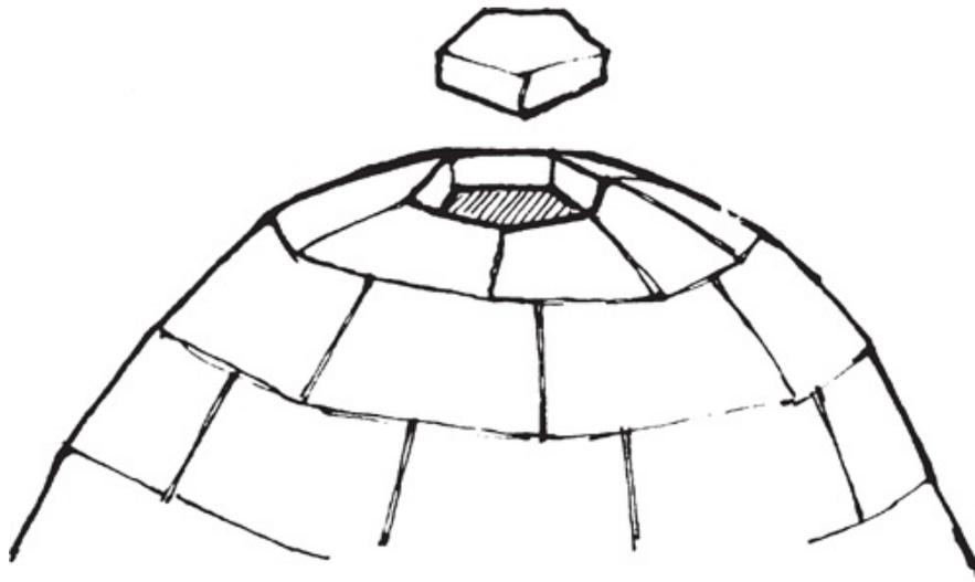
*The final block must be cut to fit — unless the space is small enough to leave for ventilation, but this last block helps to keep the structure from collapsing.*
