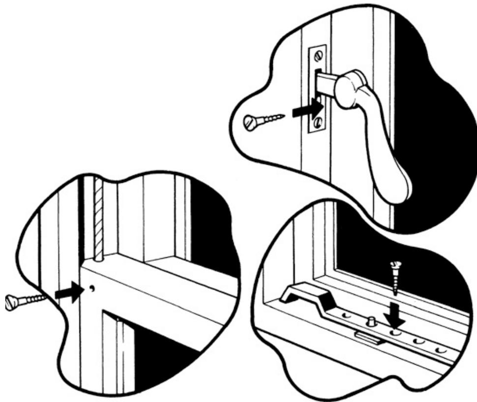
*A temporary measure, if you have sash windows, is to drill a hole through the inner sash and into the outer to hold a screw to prevent the window from being opened. Casement window catches and staybars can also be temporarily immobilized by inserting a screw.*
