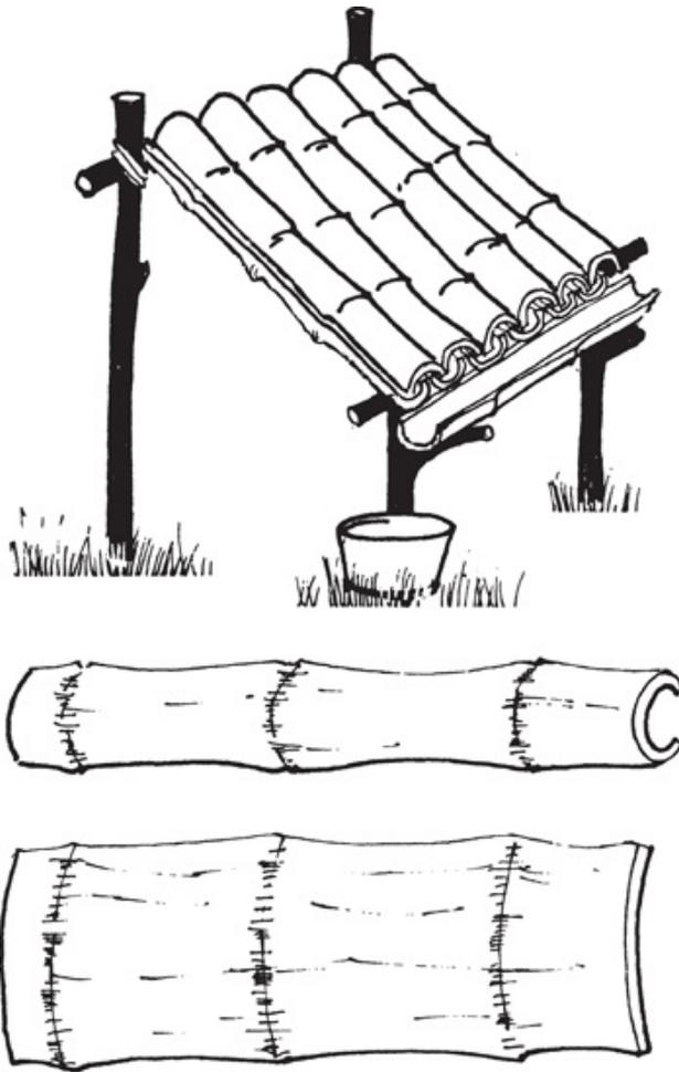
*Flatten split bamboo for smooth walls, floors or shelving by cutting vertically through the joints every 1.25cm (1/2in) or so around the circumference. It can then be smoothed out.*
