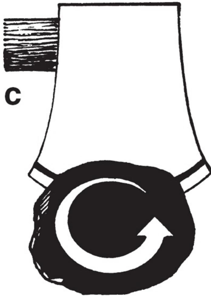
*Turn the axe over. Repeat the process circling in the opposite direction.*
