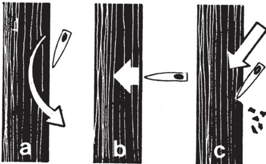
*Alternating the angle of stroke will prevent the axe from jamming. Too steep an angle will cause the axe to glance off the trunk (a). Dead-on will make it jam or be inefficient (b). Aim for 45 degrees (c).*
