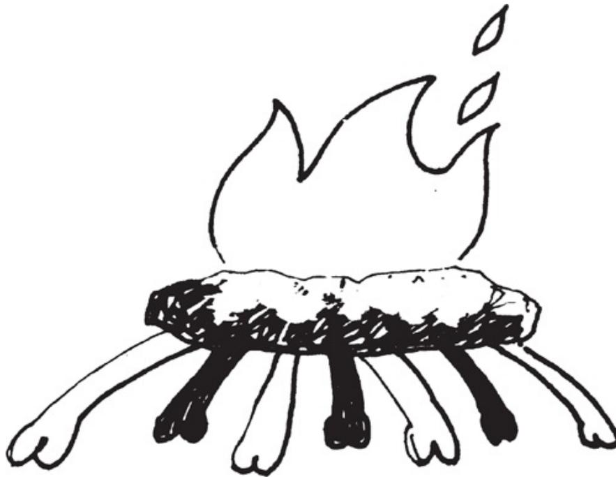
*Start flame with tinder or a candle then place a network of bones over it to support the fat or blubber. Use only a little fat at first. Unless it is surplus, burning fat means sacrificing food value, but seal blubber spoils rapidly and makes good fuel.*
