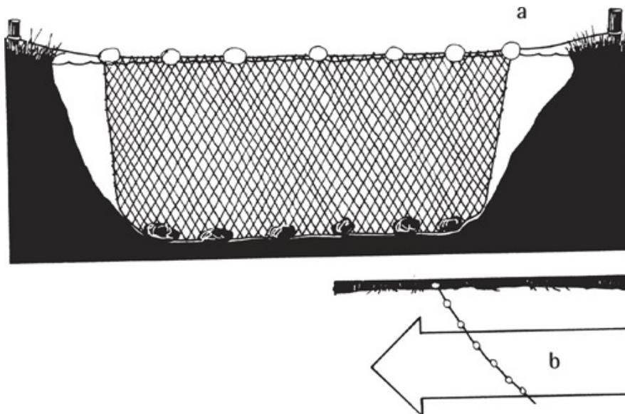
*A gill net can be anchored on each bank, (supported by weights and floats (a), or tied to fixed posts. If it is angled across the line of the current (b) there is less likelihood of driftwood building up against it.*
