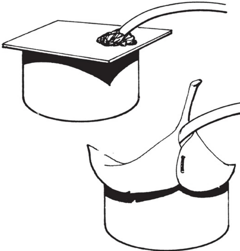
*Take a tube from a covered vessel in which polluted/saltwater, or even urine, is to boil. Set the other end under a solar still. A sheet of metal or bark, perhaps weighted down, will cover the vessel. Even a cone of leaf over the water pot will help direct the steam into the tube.*
