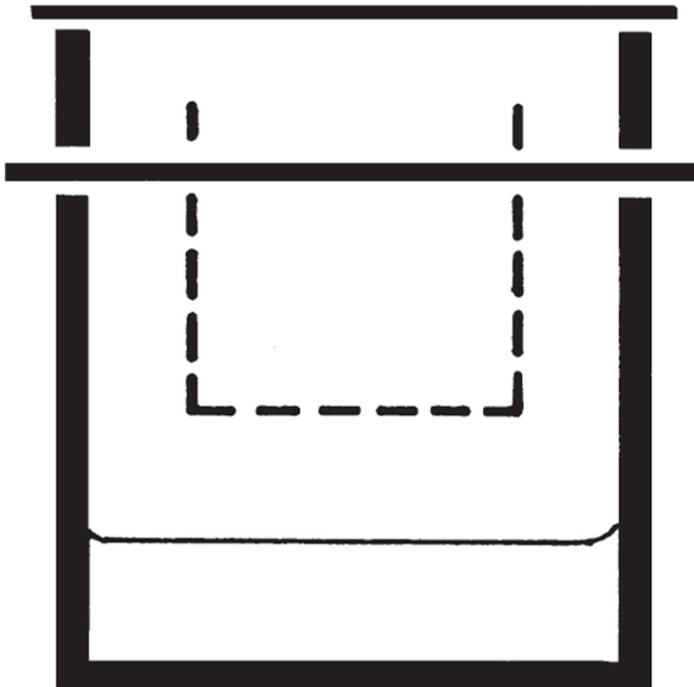
*Make a simple steamer by punching holes in a can and suspending it inside a larger can, or putting something in the bottom of the larger can to keep the inner one above the water. Cover the outer can so that steam is not dissipated, but not so tightly that it is sealed or pressure could build up and cause it to explode.*
