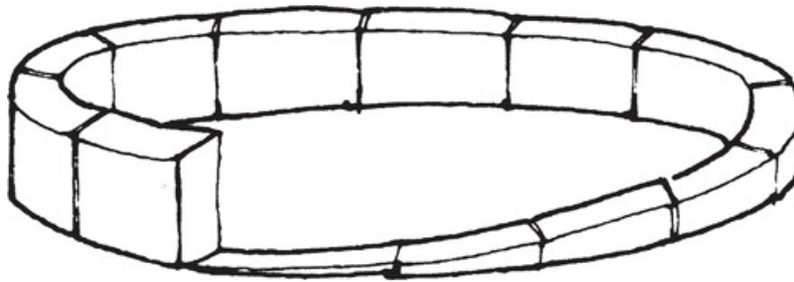
*Cutting the first course to an even spiral eases the whole process. Angle the top edge slightly down towards the centre.*
