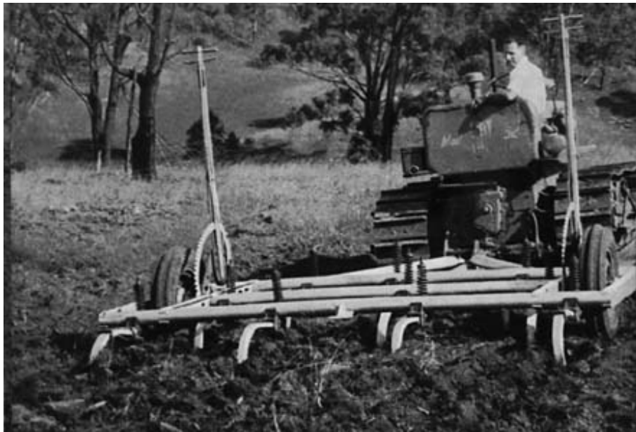
Plate 4: A 10-foot Graham Chisel Plow and Crawler used for developing steep country up to 100% slope.
