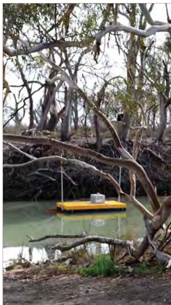
Monitoring salinity and the water table at Punkah Creek on the Chowilla Floodplain, South Australia
