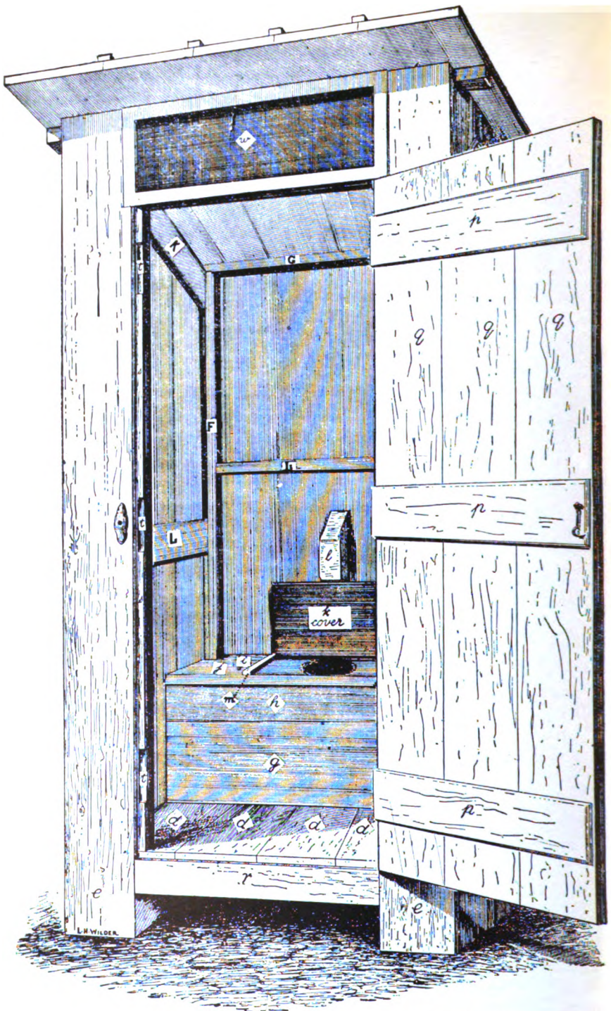
FIG. 6.—A SINGLE-SEATED SANITARY PRIVY. (STILES, 1910.)
